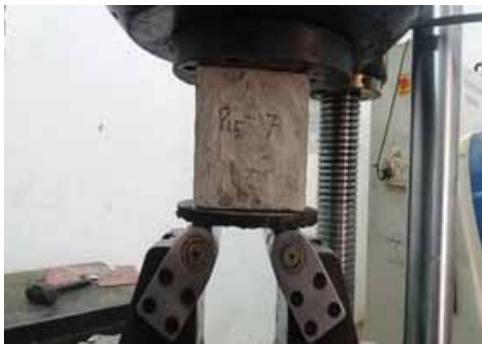
Figure 2: Compression Test Setup
