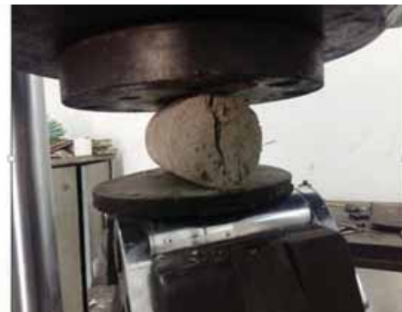
Figure 3: Split Tensile Test Setup
