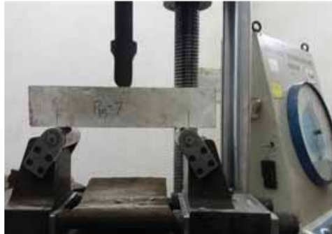
Figure 4: Flexural Test Setup
