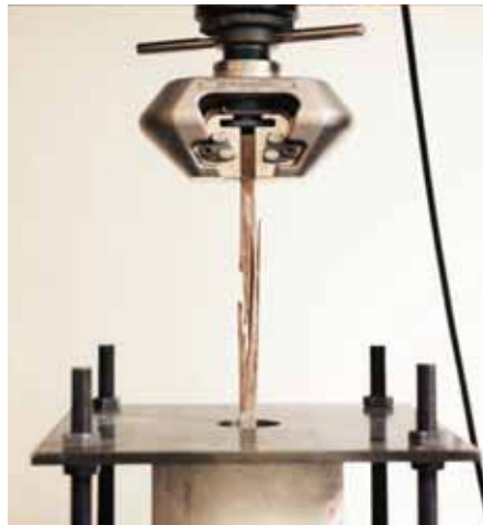
Fig 26 : Tensile Strength Test of Bamboo Image Courtesy : D.E Hebel - ETH
